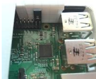
Figure 5.4 Jumper on (paired)
